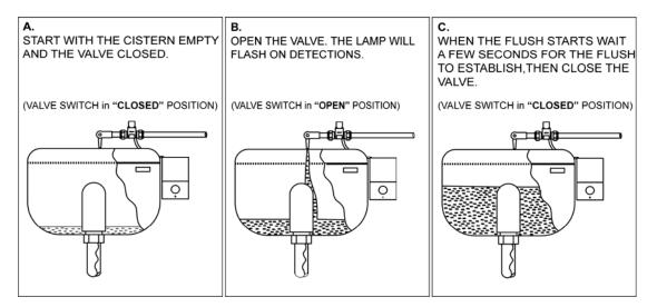
THE TIME TAKEN FOR THE CISTERN TO FILL DURING SETUP IS STORED AND USED ON ALL SUBSEQUENT AUTOMATIC FLUSHES.
