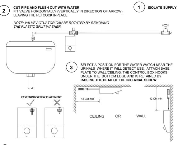
WIRE THE 1.1m CABLE FROM THE VALVE TO THE WATER WATCH CONTROLLER. IF THE CABLE IS NOT LONG ENOUGH IT CAN BE EXTENDED USING THE TWO WAY TERMINAL BLOCK PROVIDED. LEAVE A SMALL LOOP INSIDE THE CONTROLLER SO THE LID CAN BE DETACHED FROM THE MOUNTING PLATE. ATTACH THE BATTERY CONNECTOR.
